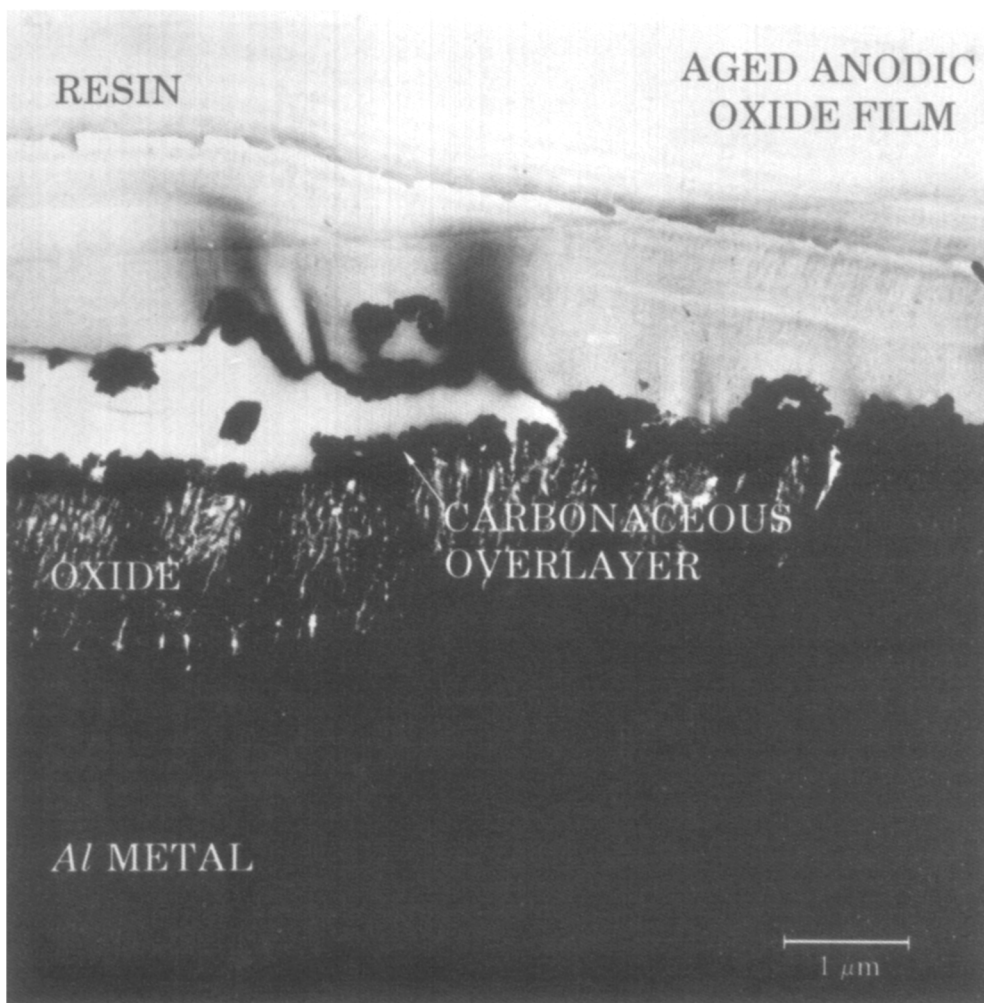
FIG. 5. TEM micrograph of Sample 4 (aged anodic alumina film).
