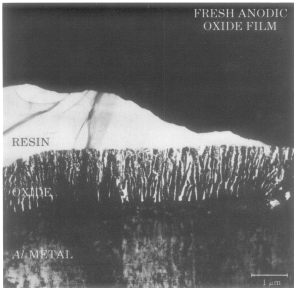
FIG. 4. TEM micrograph of Sample 3 (fresh anodic alumina film).
