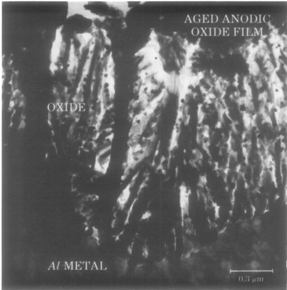
FIG. 6. TEM micrograph of Sample 4 (aged anodic alumina film) at higher magnification.
